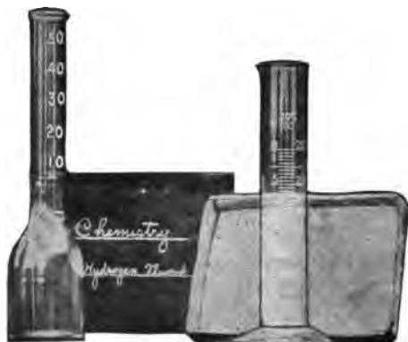
FIG. 81.—The word "chemistry" was etched with the gas hydrogen fluorid; the other words with a solution of the gas.
